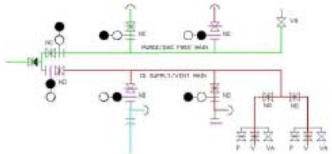
Figure 7 - Re-inerting a cargo tank after access. IG Supply/Vent main contains HC, Purge/Gas free main contains IG. Air is vented out via a portable hose.
