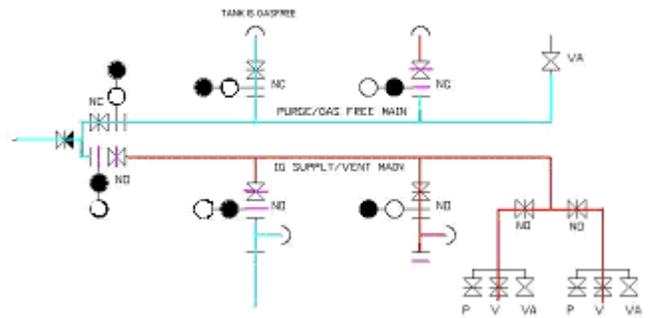
Figure 6 - FPSO gas free cargo tank isolation during access. IG Supply/Vent main contains HC, Purge/Gas free main contains air.
