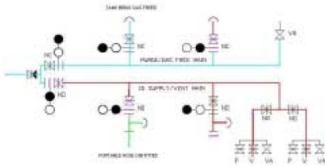
Figure 5 - FPSO cargo tank gas freeing with air supply via Purge main. IG Supply/Vent main contains HC, Purge/Gas free main contains air. IG is vented out via portable hose. Other tanks vent via IG vent main.
